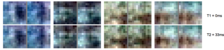
Fig. 1. Gradient Ascent Visualizations. Shown are four neurons’ receptive fields from Layer 1 of our first self-driving network. Each neuron filter is divided into sub-filters, with one sub-filter per camera, per input frame – hence the 2x2 layout per neuron filter. These filters appear sensitive to optical flow and stereoscopic disparity.
